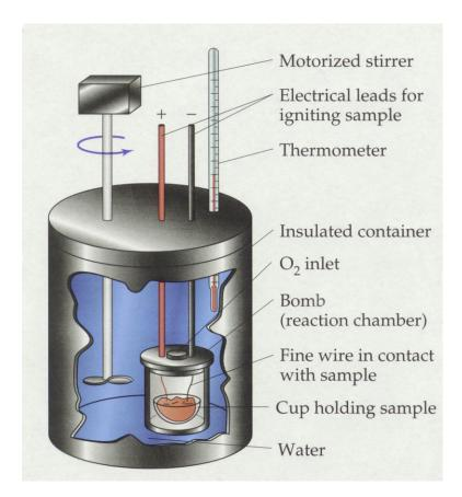
The rise in temperature is recorded and a calculation is used to work out the amount of energy released. We can carry this out in the school laboratory using a simpler set up, however not as accurate as the bomb calorimeter.
