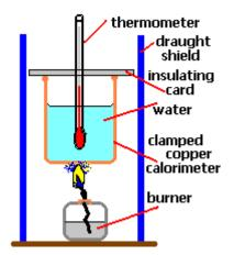
The fuel is burned and will cause the temperature of the water to rise. We then use the following equation to calculate the amount of heat energy released.
